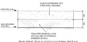
**BUILDING BULK EXCAVATION DETAIL**
